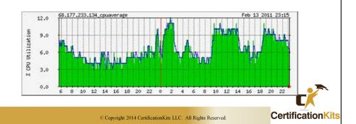
The **show processes cpu** command displays overall router CPU utilization as well as the CPU utilization of each of the processes running on the router. The output CPU utilization for the past 5 seconds, past 1 minute and past 5 minutes.
